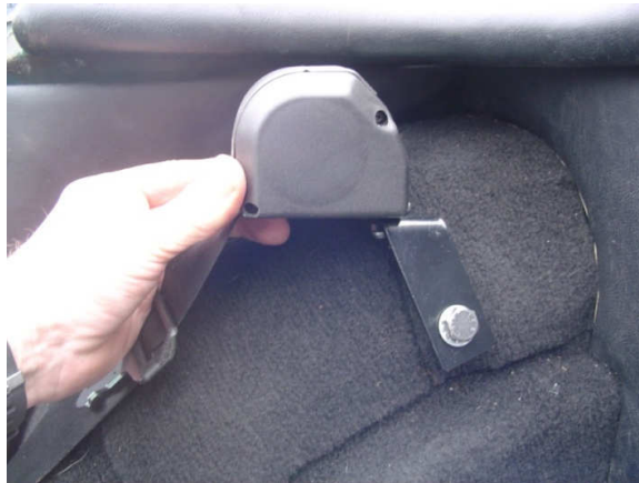
Fig9 Final Installation NB Inertia Mechanism mounted horizontally
