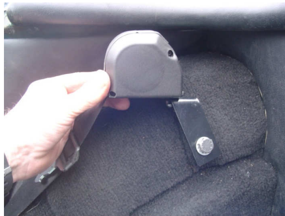
Fig9 Final Installation NB Inertia Mechanism mounted horizontally
