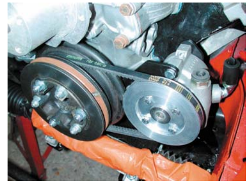
Belt-driven mechanical pump on MGB GT V8 type installations
