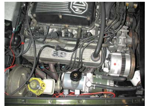
RV8 uses electro-hydraulic pump mounted on the offside fitch panel
