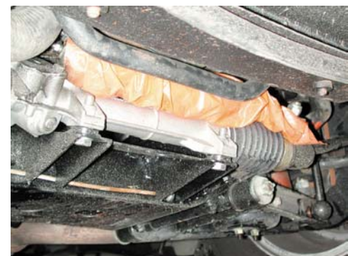
Modified steering rack mountings with steering rack fitted to the MG RV8 front crossmember. A similar installation is used in the H629 kit for MGB GT V8s fitted with the Performance MGB Complete Front Axle Assembly (derived from the MG RV8 item)
