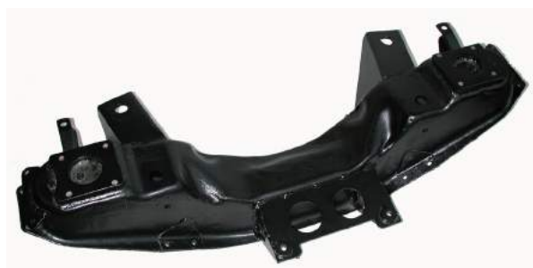
Pre-modified crossmember, with rack brackets welded in position, supplied on exchange basis
