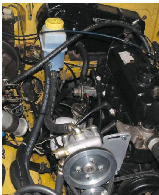
Rubber bumper 1976 onwards installation, featuring belt-driven pump powered from double alternator pulley
