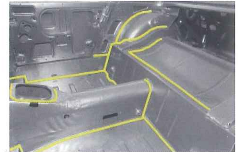
Tunnel and rear body Apply to both sides of the tunnel, down into the footwell, rear floor and rear inner wheel arches.
